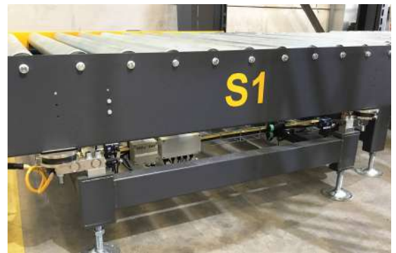
Weighting cell under roller conveyor
